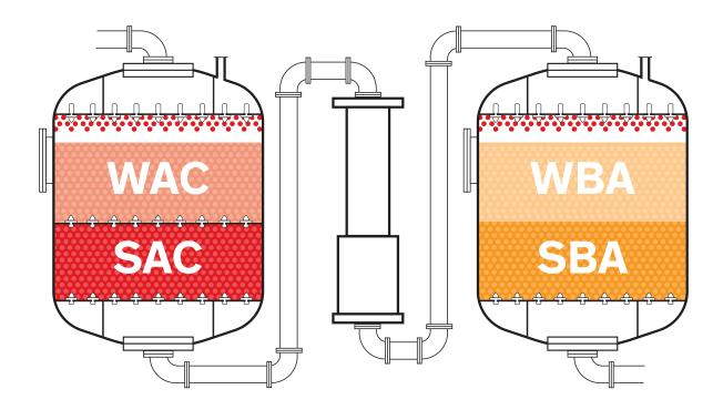
Weak resins are well-suited for use with strong resins to improve overall efficiency and throughput of a demineralization system. Layered beds using weak and strong resins in a single vessel allows for significant capital cost and footprint savings compared to using the resins in two separate vessels.
